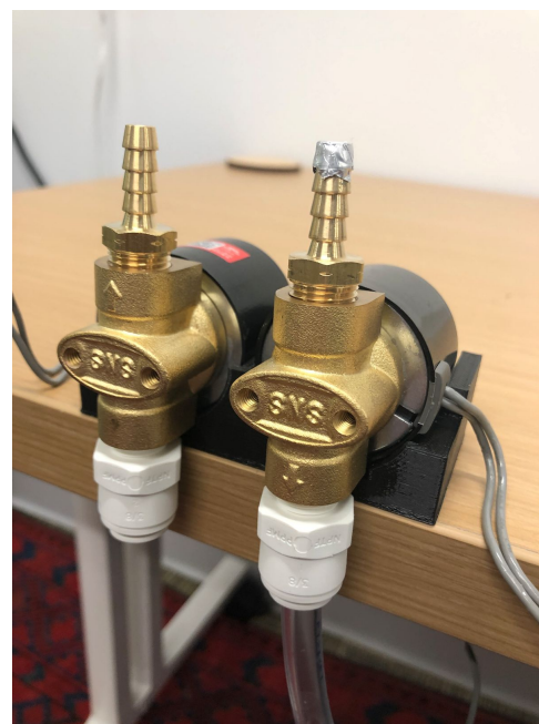
Figure 1: Both solenoid valves side by side in the valve cradle. The valve on the right has the tinfoil covering with a 1mm hole in it (hole not shown)
